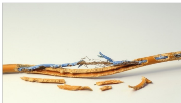
Electrical cables with damaged insulation
